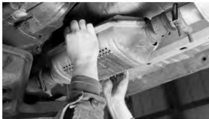
Removing a catalytic converter
