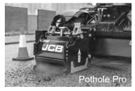
perimeter of the hole neatly to allow a watertight repair, and then it brushes away and collects the debris afterwards. Highways teams just need to lay and compact asphalt into the prepared hole to complete the repair.
